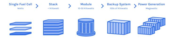
Individual fuel cells are coupled into stacks to make larger systems. In batteries, leads (wires) are attached to the electrodes in each cell. Fuel cell engineers have a more difficult challenge: they have to design systems to deliver hydrogen and oxygen gases to each cell in the system. (Adapted from <u>Bloom Energy</u>)
