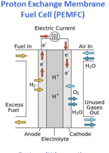
Protons (H<sup>+</sup>) cross the electrolyte to the cathode
