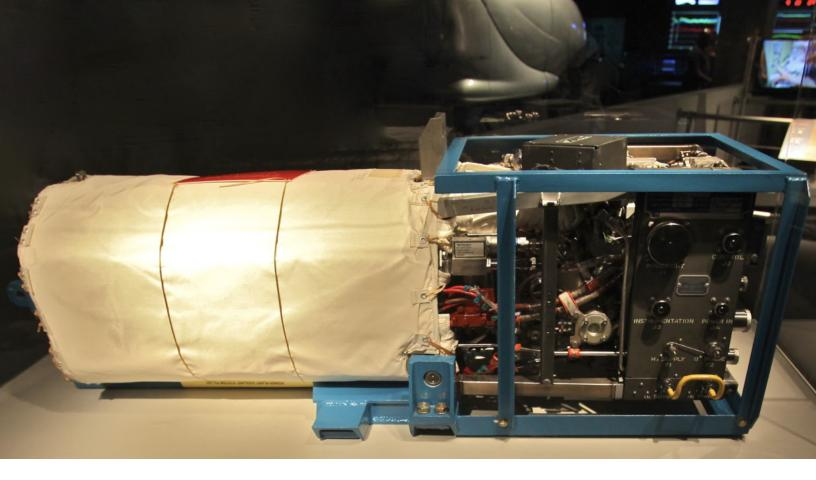
A fuel cell assembly from the Space Shuttle Orbiter, retired in 2012. So analog! <u>Photo by Steve Jurvetson</u> under CC
