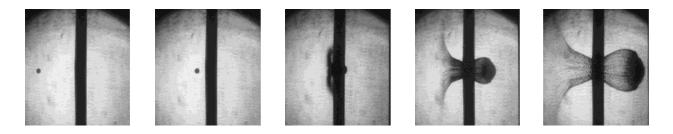
Projectile impacting a thin aluminum plate at 7,000 m/s. The particle disintegrated and created fragmentation on the backside despite not penetrating the plate. Image credit: NASA, Public Domain
