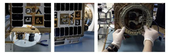
SCOUT-vision payload (noted by high-lighted areas) launched by SpaceX in June 2021 onboard orbit Fab's Tenzing-001 tanker. Image credit: SCOUT [27]
